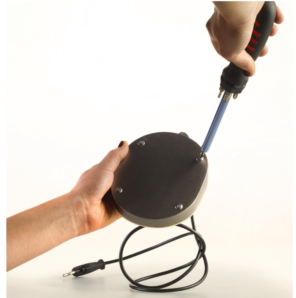
THE TINY INDUCTION STOVE IS EASILY TO REPAIR, BECAUSE OF ITS REMOVABLE BOTTOM COVER
