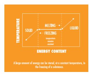
This means that the vapor compression cycle only needs to run once a day to freeze the phase change material, which will then stay cold for the remainder of the day.
