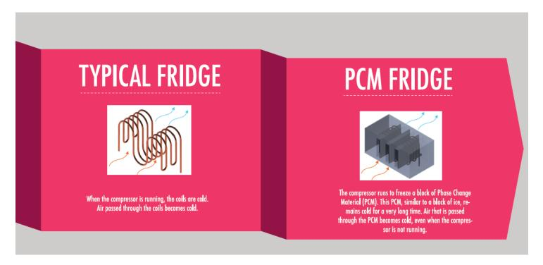
By contrast, the Ecofridge uses Phase Change Materials (PCMs) to store energy from a standard vapor compression cycle. A large amount of energy can be stored, at a constant temperature, when you freeze a substance. The cold thermal energy stored in the PCM can then keep the coils cold for a designed amount of time (1 day).
