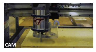
I used the CAM workspace to move from digital to physical. In the image above, a CNC router is following a toolpath created in Fusion to cut out one of the tumbler petals or handles. This was immensly helpful because it allowed me to create full scale prototype pieces very quickly. From seeing and holding these 1:1 scale pieces I got a sense of size and feel for the product and made tweaks in the model accordingly.
