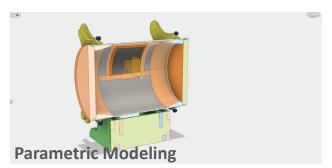
I used parametric modeling, not direct. Most of the components in my model appear more than once in my assembly. By using the timeline feature, arrays, and mirrors, I was able to change one component's parameters and have that change be reflected in all of the dependent bodies.
