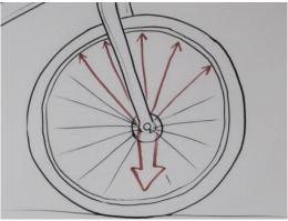
The weight of the rider at the axle is pulling down on the top of the wheel. So tension is being substituted for compression. If the spokes were being pushed on, they would certainly buckle, because they are 150 times as long as they are wide.
