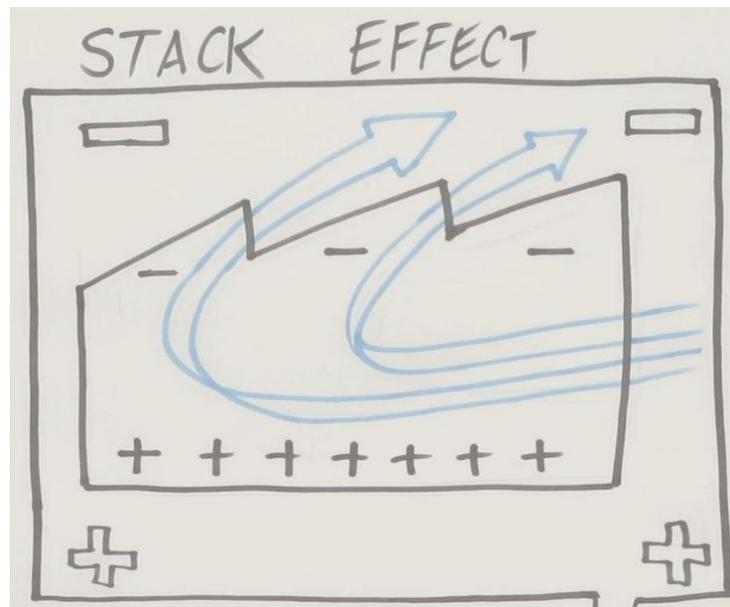
Wind and heat make air pressure lower farther from the ground. Higher pressure air then wants to move there, so if you have windows at the top and the bottom, air will naturally flow upwards with no fans needed!
