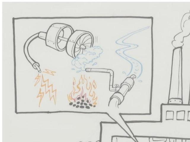
This converts coal's chemical energy to heat energy, then to mechanical energy, then to electrical energy. That's a lot of conversions, and the total efficiency is about 35%.
